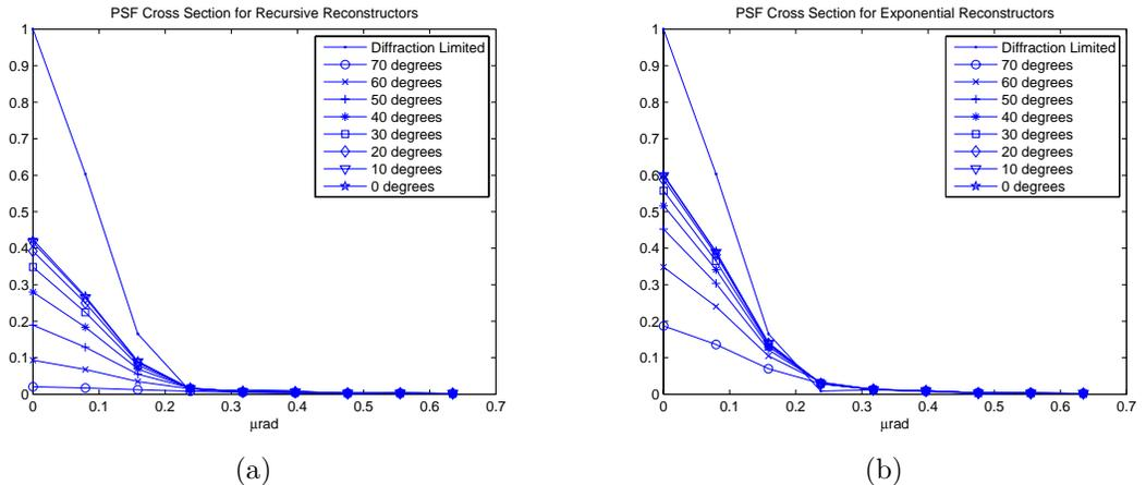
Figure 3: (a) Average PSFs for the recursive reconstructor as a function of  $\theta_Z$  for the MAUI3 turbulence profile; and (b) average PSFs for the slope discrepancy reconstructor as a function of  $\theta_Z$ .
