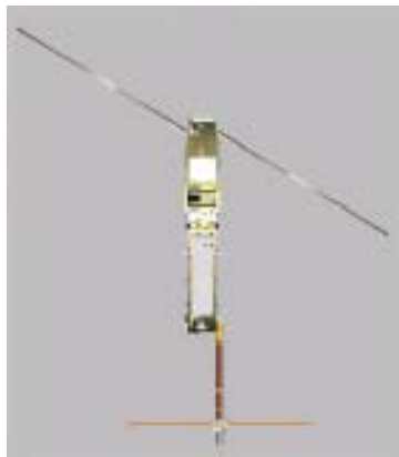
Fig. 4. Side view of FORMOSAT to illustrate the solar panel orientation to the spacecraft body
