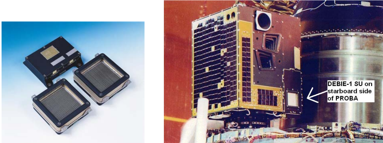
Fig. 5: Left: the DEBIE-1 flight model with 2 sensors units. Each SU area is 10 cm x 10 cm. Right: One SU of DEBIE-1 is visible at the bottom right corner of the PROBA satellite.
