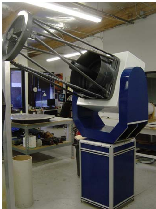
Fig. 4. Lightweight telescope (in black) mounted on portable AO system (white) and lightweight mount (blue fork).
