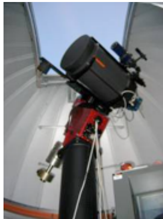
Figure 2: The DRDC SSO as seen from inside. The mount, optical tube, and CCD camera are in the center, while the environmental enclosure containing the computer and networking equipment is in the lower right.
