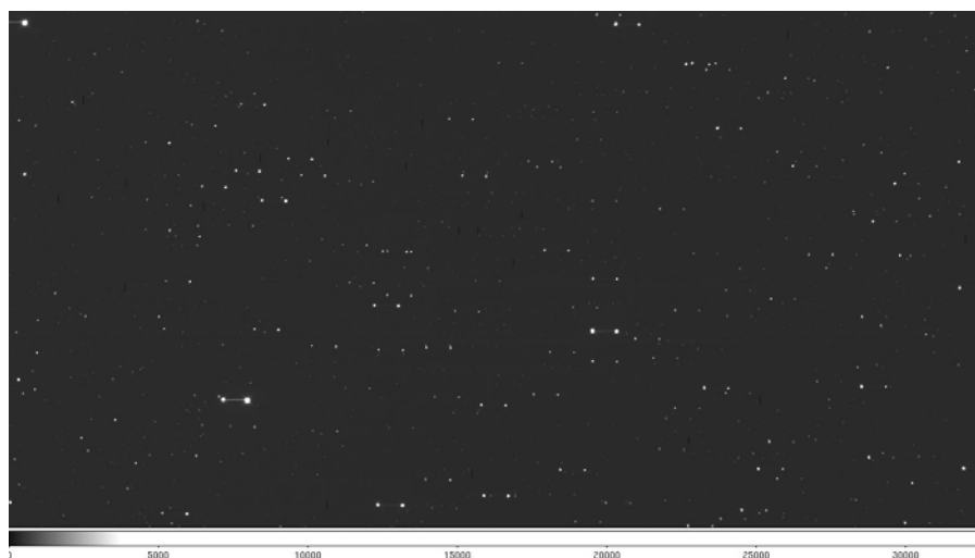
Fig. 10. A modulated CCD image can be used to embed accurate time hacks into image data. Multiple displacements with unequal intervals allow determination of the direction of motion of a satellite leaving a track in the image. The fields of view of multiple telescopes can be angularly registered by the star images, and registered in time by the displacements. These data are sufficient to derive a terrestrial parallax and a range estimate.
