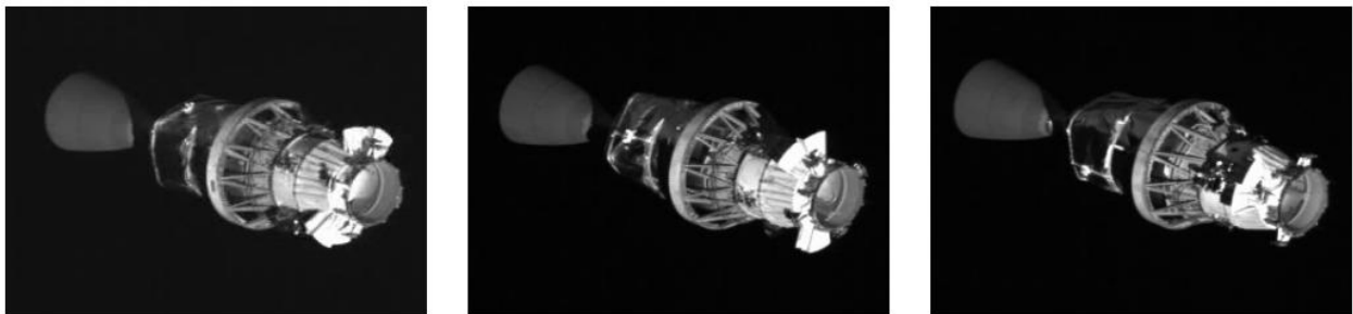
Fig. 1: A subset of the images of a rocket body taken from the XSS-10 satellite. The full sequence has 25 images and depicts over 720 degrees of rotation primarily about the rocket body's main axis.
