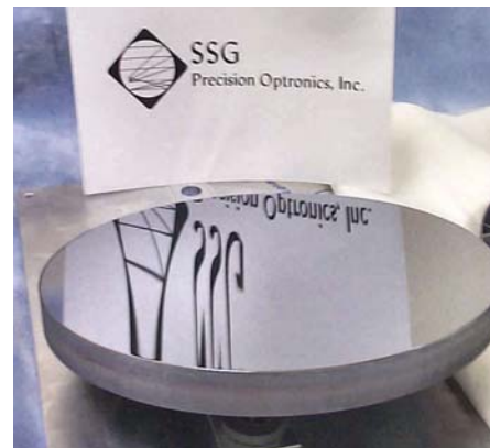
Fig. 7. Photo of Silicon Coated SiC Aspheric Finished Optic
