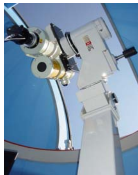
Fig.2(a). Eccentric elbow-type mount, 25cm and 16cm telescopes.
