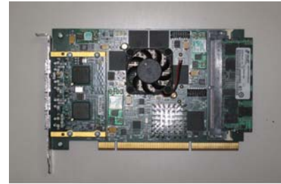
Fig.9. FPGA board H101-PCIXM manufactured by Nallatech
