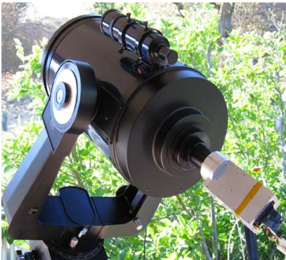
Fig. 18: Small (25 cm) telescope tests with sealed tube 18mm XS sensor (uncooled), as a testbed for imaging with photon event time tagging.
