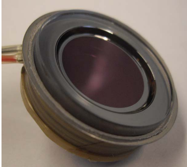
Fig. 3. 18 mm sealed tube sensor using the 22 mm cross strip anode shown in Fig. 2. The tube has a SuperGen-II photocathode giving a broad wavelength range coverage.
