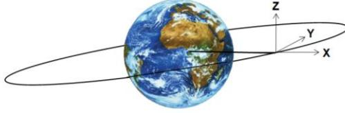
Fig. 2. LVLH coordinate system.
