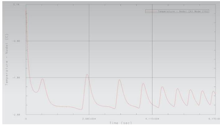
Fig. 5 Transient temperature of the Camera Lens
