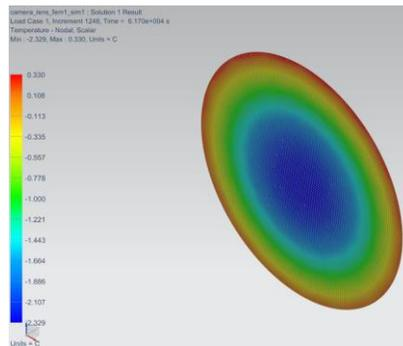
Fig. 4 Temperature Contours Mapped Onto Structural Thermal Model
