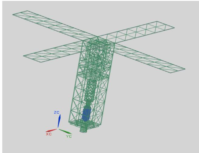
Fig. 1 Thermal Finite Element Model of Cubesat and Camera Payload
