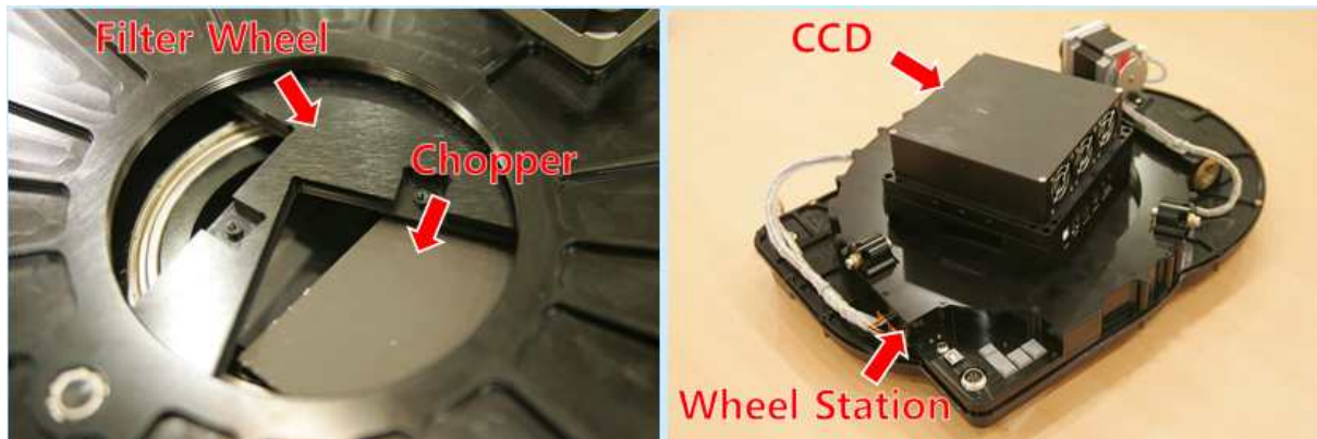
Fig. 5. Filter wheel and chopper (left) and wheel station and CCD camera (right)
