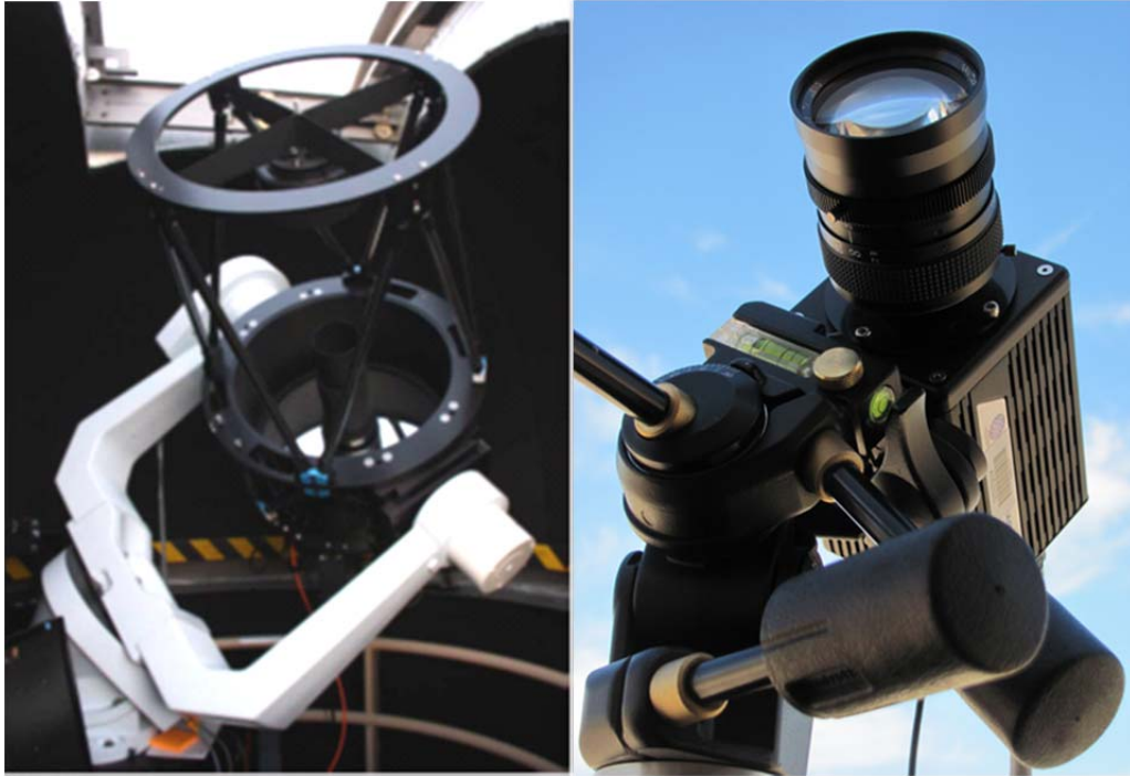
Figure 1: (a) AFRL/RH 17-inch telescope inside the dome. (b) AFRL/RD EM-CCD based camera
