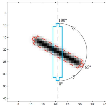
Figure 1. Rotation of filter perfectly matching an example of a streak with length 21 pixels.
