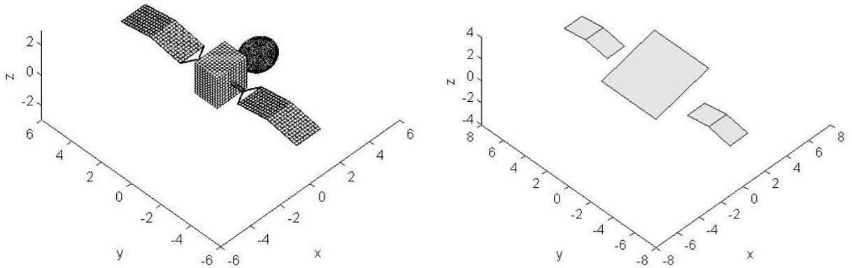
**Figure 1 –Satellite models (a) full, and (b) simplified**
