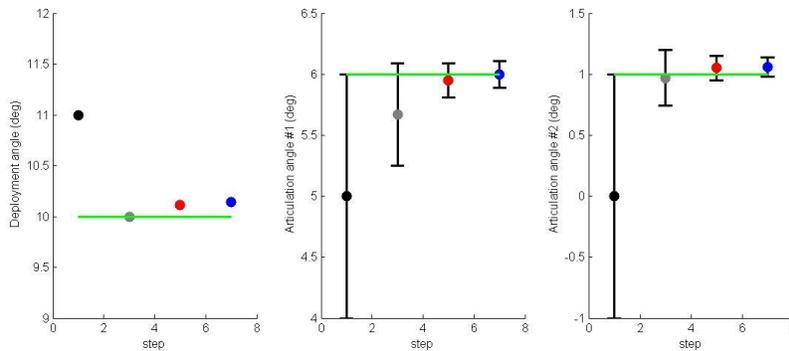
**Figure 7 – Solar Panel deployment angle, and articulation angles for various steps in process. Truth values shown as horizontal green lines.**
