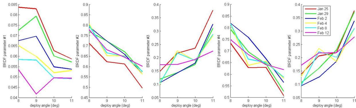
**Figure 3 – BRDF values as function of deployment angle from step 3 analysis of training set.**
