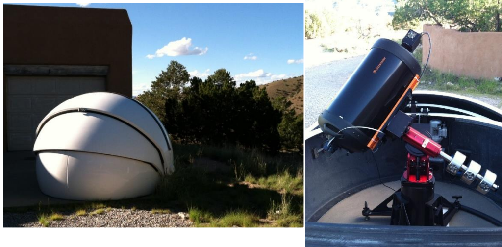
Figure 2. The northern JTMA Proof-of-Concept LEO SSA Optical Systems shown enclosed and opened to the sky awaiting twilight. The optical systems are 14" Celestron Schmidt-Cassegrain telescopes with Hyperstar prime focus wide field correctors installed. A FLI ML-16070 interline CCD provides a 3^\circ \times 2^\circ field of view with 2.25" pixels and can be read out at 1 Hz with no deadtime between frames. The systems are enclosed in 7ft Astrohaven clamshell domes.
