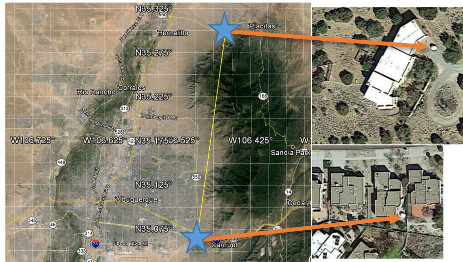
Figure 1. JTMA's Proof-of-Concept LEO SSA Optical Systems are separated by 27 km enabling them to simultaneously observe the same volume of LEO and obtain range estimates based on parallax for objects detected with both systems.
