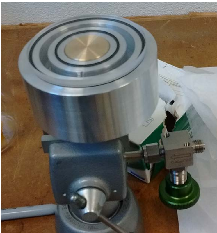
Figure 6 Small "vacuum wallet" for in vacuo electron aging and characterization of polymer samples. Initial testing shows that the double o-ring seal maintains vacuum for >2 months. The brass sample mounting surface (center) is spring loaded to ensure good contact between the aged polymer and the CaF 2 window surface in order to minimize multi-surface reflections. Planned upgrades include a small inline pressure gauge in order to characterize the effects of pressure quantitatively.
