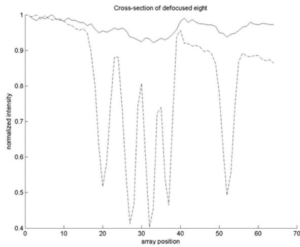
**Fig 8: Cross-section of the defocused section of the test grid showing the blurred spectral features. The solid line is the blurred spectral features due to the focus error. The dashed lines show the focused spectral features.**
