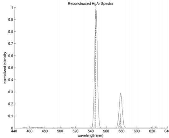
**Fig: 14 Reconstructed spectra of the Hg(Ar) source with the finer 5nm filter sampling. The solid line shows that the spectral lines at 546nm and 577/579nm are resolvable, and are closer to the spectral lines of Hg(Ar), shown in the dashed lines.**
