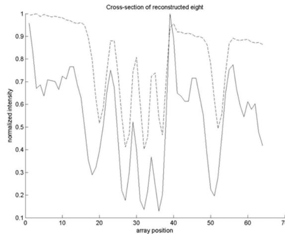
**Fig 11: Cross-section of the reconstructed section of the test grid. The solid line shows the spatial features are now resolvable and compare well with the same features in the focused section of the test grid. The dashed line shows the focused spatial features.**
