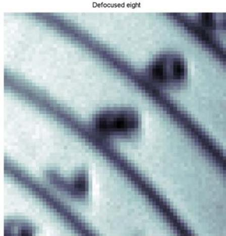
**Fig7: Defocused section of the test grid containing the spectral features.**
