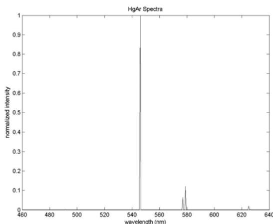
**Fig 4: The spectra of the Hg(Ar) source.**
