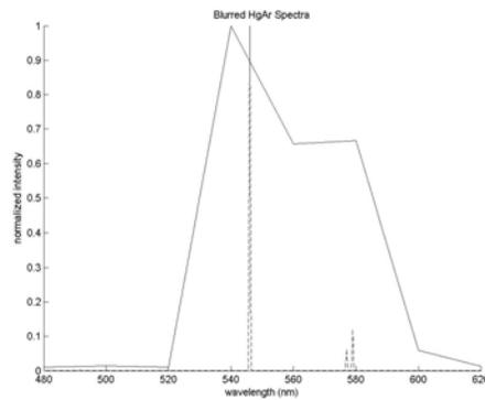
**Fig 9: The blurred spectra due to the coarse 20nm filter scan. The solid line is the blurred spectra, the dashed lines are the spectral lines of Hg(Ar).**
