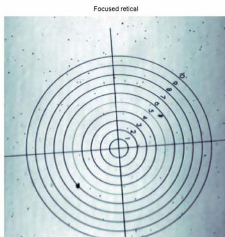
**Fig 3: The test grid collected at a filter setting of 546nm.**
