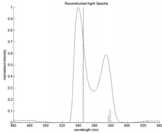
**Fig 12: Reconstructed spectra of the Hg(Ar) spectral source. The solid line shows that the spectral lines at 546nm and 577/579nm are now resolvable, but are slightly shifted from the spectral lines of Hg(Ar), shown in the dashed lines.**
