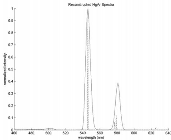
**Fig: 13 Reconstructed spectra of the Hg(Ar) source with the shifted filter sampling. The solid line shows that the spectral lines at 546nm and 577/579nm are resolvable, and are closer to the spectral lines of Hg(Ar), shown in the dashed lines.**
