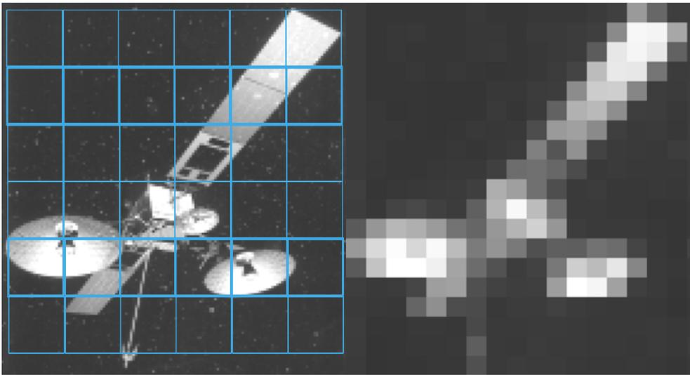
*Fig. 4: Notional Pixel Sizes for VNIR Collection of TDRSS*
