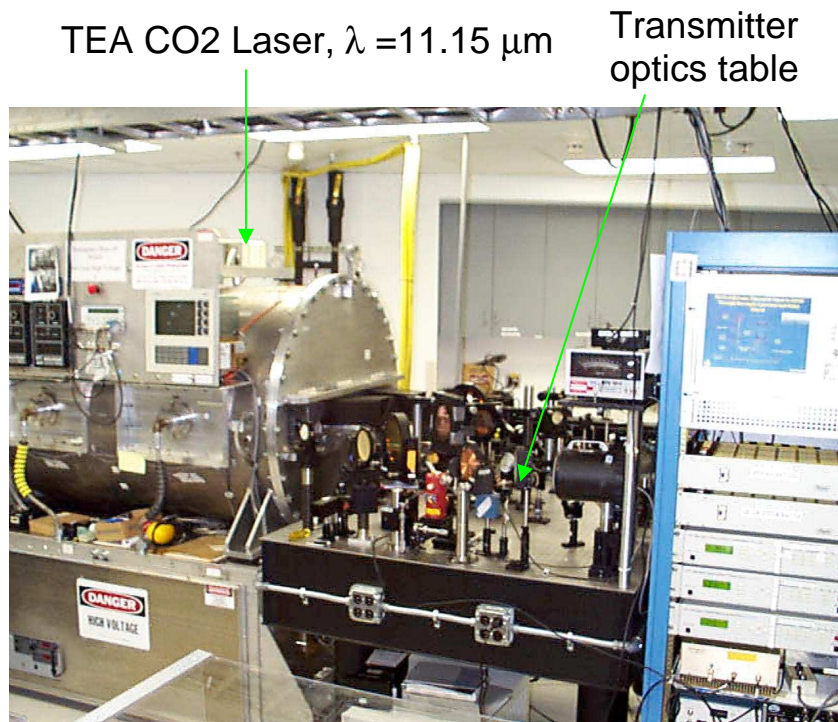
Figure 1 The TEA laser is the large chamber indicated. The bench in front of it holds transmitter optics and the seed laser.
