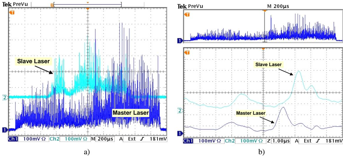
**Figure 7. Lasing traces of the of Slave and Master cavities at ALTS-target distance 1.5 km.**
