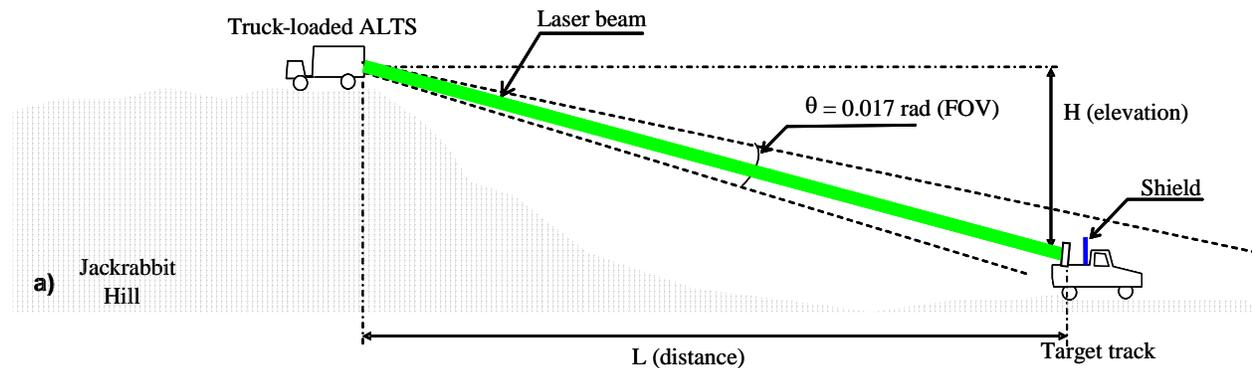
Figure 4. The ALTS deployment scheme
