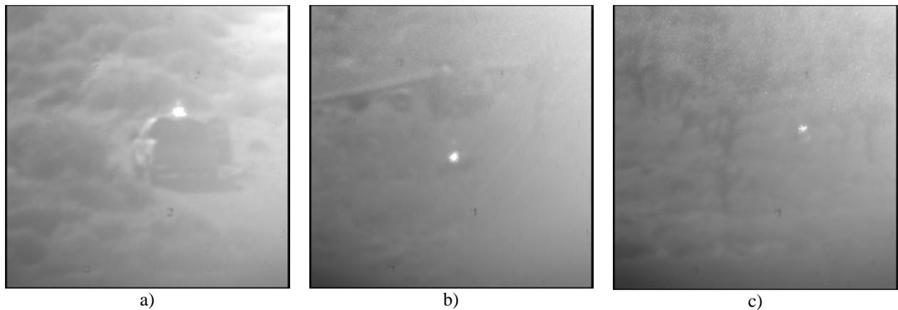
**Figure 6. ALTS images with lasing spot at the range: a) 1.5 km; b) 3.5 km; c) 6.38 km**
