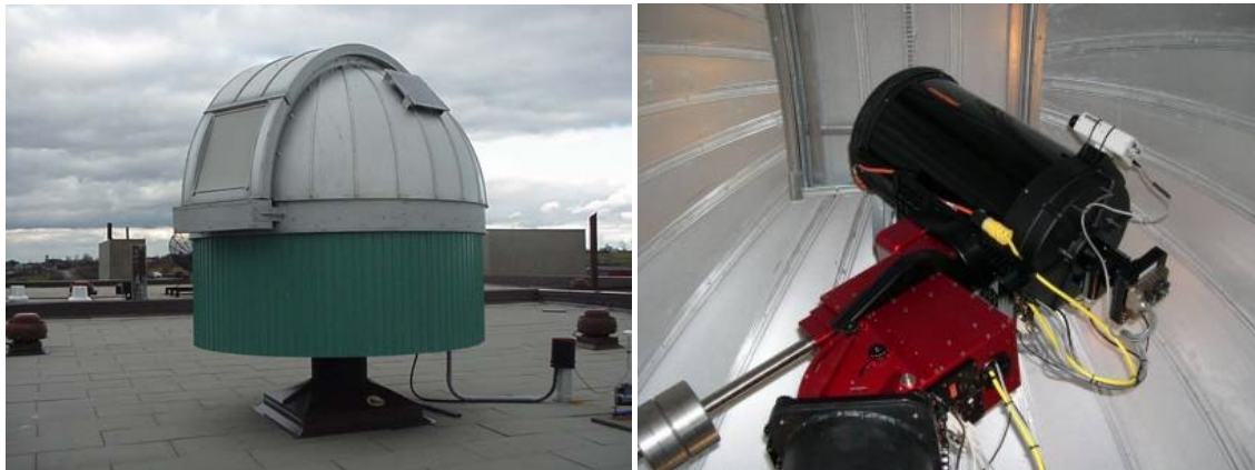
Fig. 1. Dome, and Optical Tube, Robotic Mount, and Camera Assembly of a CD Telescope
