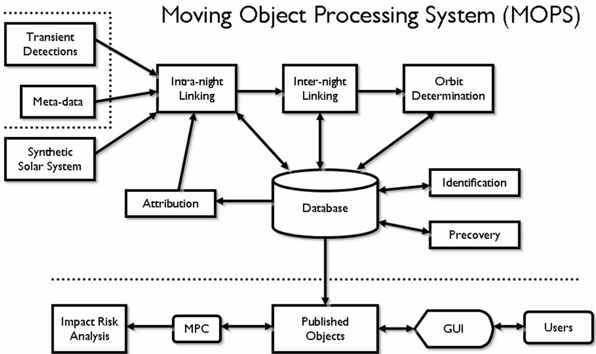
Figure 1 - Moving Object Processing System concept of operations. Data in the upper left region surrounded by dotted lines is provided by the IPP. Systems below the horizontal dotted line are not part of the MOPS.
