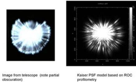
**Figure 9. A Comparison of Measured and Theoretical PSFs**
