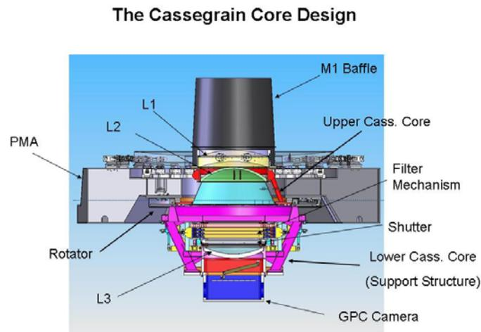
**Figure 5. The PS1 Cassegrain Core**
