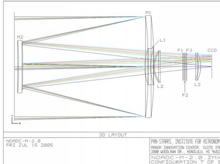
**Figure 1. The PS1 Optical Layout**
