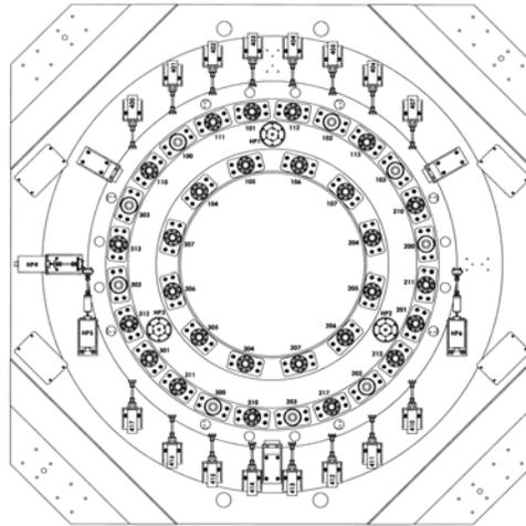
**Figure 3. Primary Mirror Cell Actuator Layout (with permission from EOS Technologies)**
