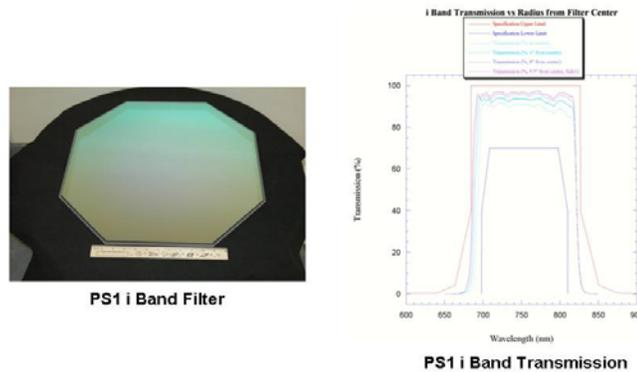
**Figure 10. The PS1 i Band Filter**
