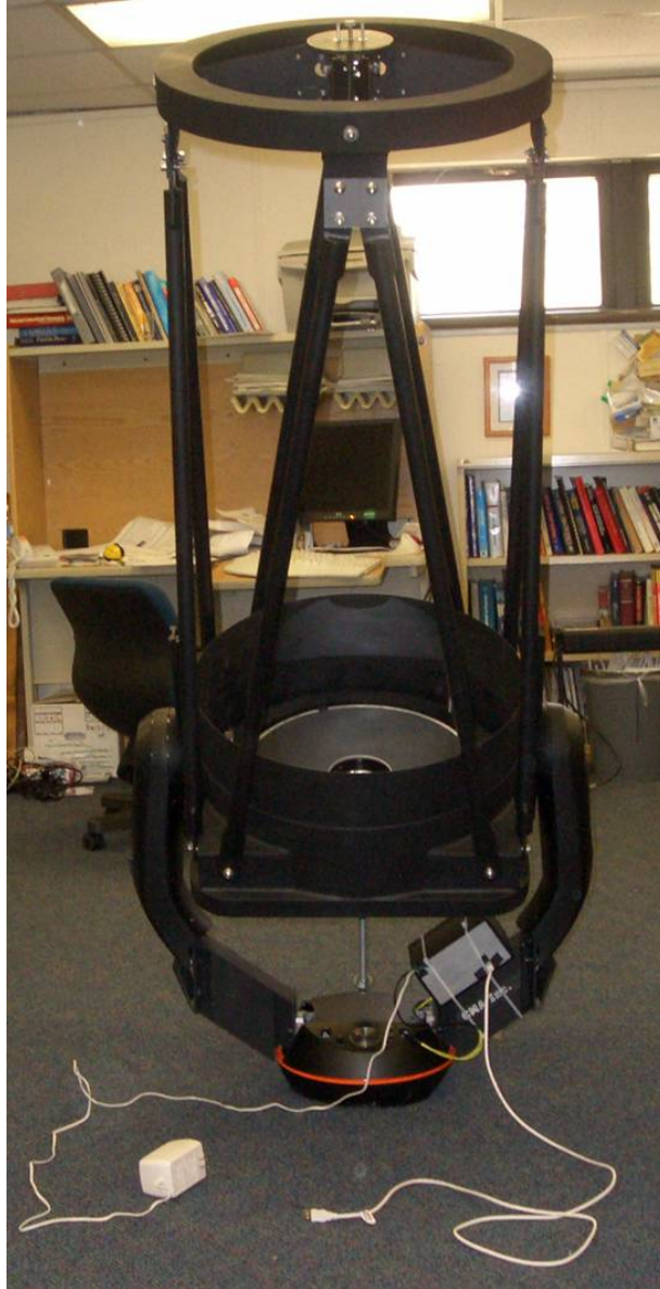
Figure 3: the 16" OTA mounted on the 8" Celestron mount.
