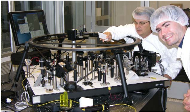
Figure 9. Lab engineer Daren Dillon and graduate student Mark Ammons perform final alignments on the Villages instrument in the LAO. Hartmann sensor readout is shown on the display behind them.
