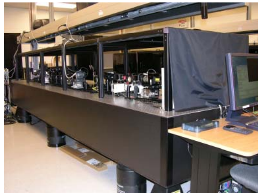
Figure 5. MCAO/MOAO Testbed showing major element and highlighting its reconfigurability for multiple guide star wavefront sensors, closed loop (MCAO), and open loop (MOAO) architectures
