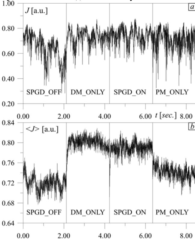
**Fig. 3. Characteristic examples of metric  $J$  time dependence corresponding to a single (a) and averaged (b) adaptation trials composed of four adaptation phases. The pinhole size is equal 150 micron. Light source was Antares at elevation angle 16 deg. The AMOS AO system was on.**
