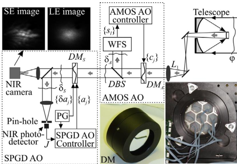
**Fig. 1. Notional schematic of the cascaded AO imaging system and examples of short-exposure (SE image) and long-exposure (LE image) images of a star (Antares at 14 deg) obtained with NIR science camera without AO systems. Pictures at right bottom show two adaptive mirror types used in the SPGD AO system: 13-electrode bimorph DM (left) and 49-electrode pocket mirror (PM).**
