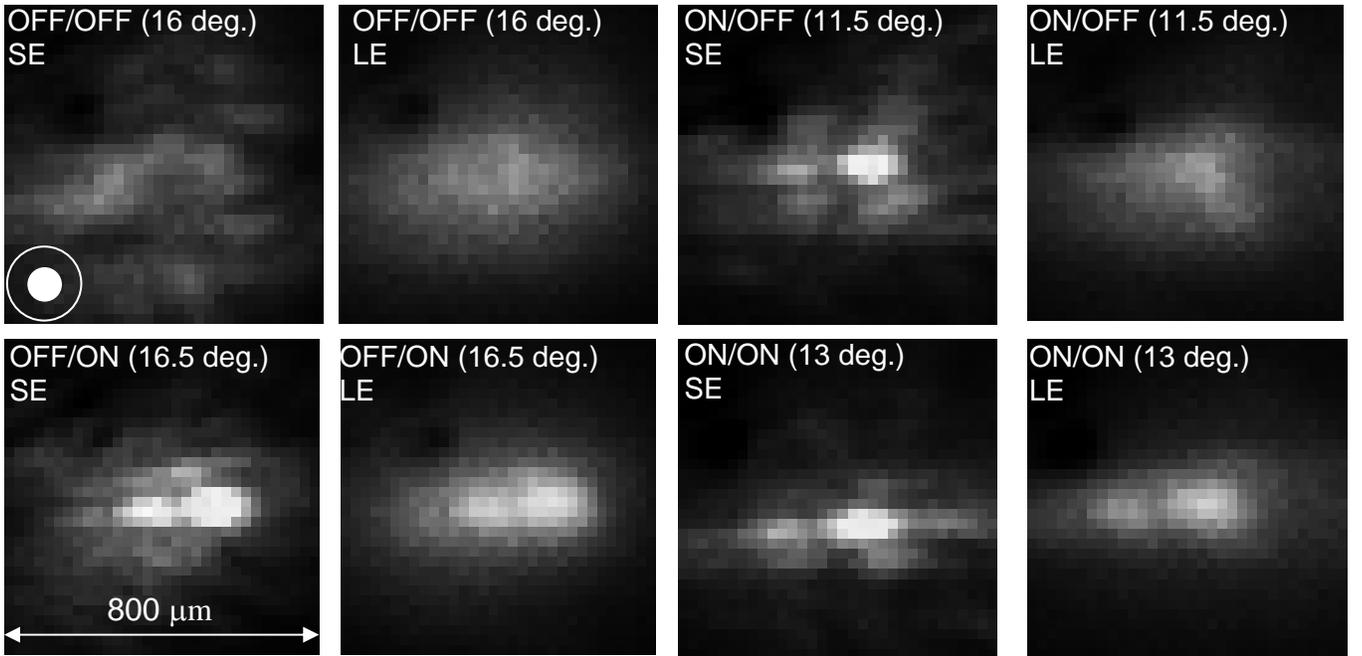
**Fig. 6. Short- (SE) and long- (LE) images of the star Antares at low elevation angles (numbers in parentheses) obtained in the cascade adaptive optical system with operational regimes (OFF/OFF; OFF/ON; ON/OFF and ON/ON) on May 18, 2007. The diffraction-limited image and the pinhole sizes are shown in the upper left photo by white circle and ring respectively.**
