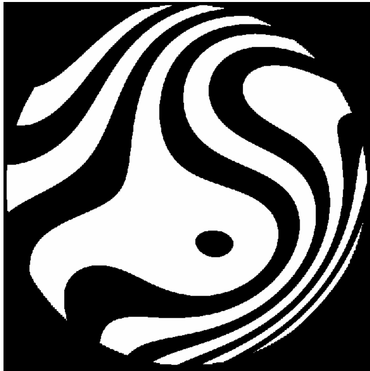
Figure 3 – Sample fringe pattern of atmospheric turbulence for the phase screen to be applied to the SLM.
