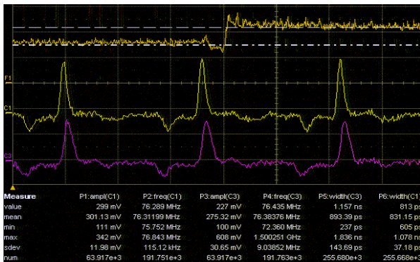
Fig. 6. 1319 nm modelocked pulse width shift during instability period.
