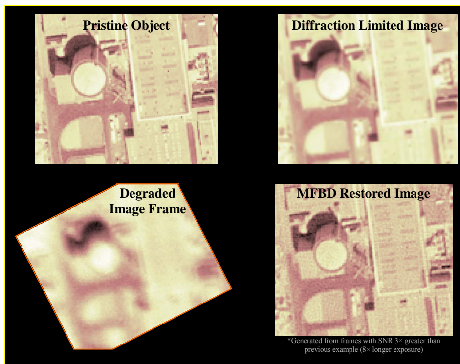
Figure 2. Comparison of Multi-Geometry MFBD restored image quality to original measured data and the diffraction limited image shows recovery of at least if not better than diffraction limited quality.
