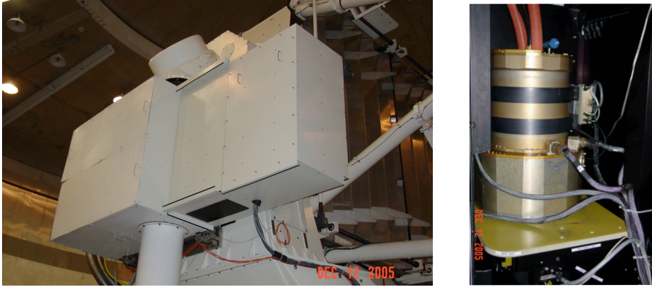
Fig. 3. Two photographs showing BASS's accommodation on the AEOS telescope. The left-hand photo shows the BASS enclosure (right), conjoined with the long wavelength IR imager (left), with the 3.6 m primary mirror behind and to the right. The right-hand image shows the BASS dewar mounted inside the enclosure (cover removed for clarity). Below the sliding shelf that BASS rests on is mounted the CCD camera that is used for real-time telescope guiding on targets.
