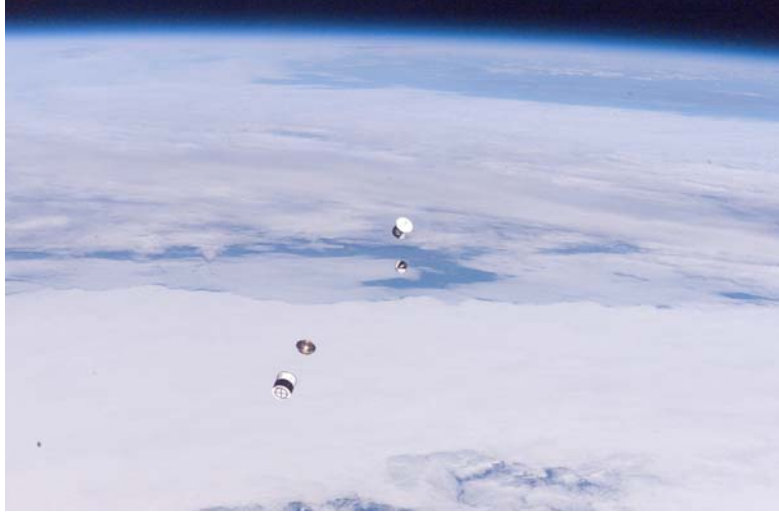
Fig. 1. Deployment of ANDERR during STS-116 on Dec. 21, 2006. From bottom to top the objects are: the ICU lower cylinder ( 29663, with MAA spacecraft (29664) still inside), the ICU avionics deck (29666), the FCal spacecraft (29667), and the ICU upper cylinder (29665).
