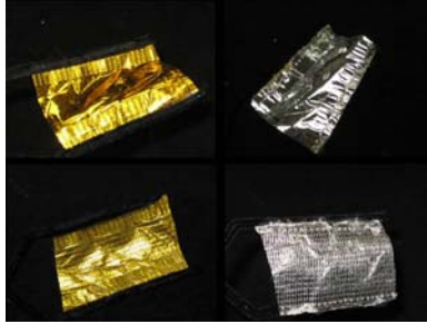
Fig. 4: Top left and right image of space-facing copper colored Kapton with aluminized backing. Bottom left and right image of spacecraft copper colored Kapton with aluminized backing.
