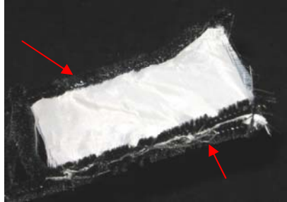
Fig. 5: Image of interior layer of MLI made of Dacron or Nomex Netting. Image enlarged to illustrate pipe cleaners used to hold all pieces taut.
