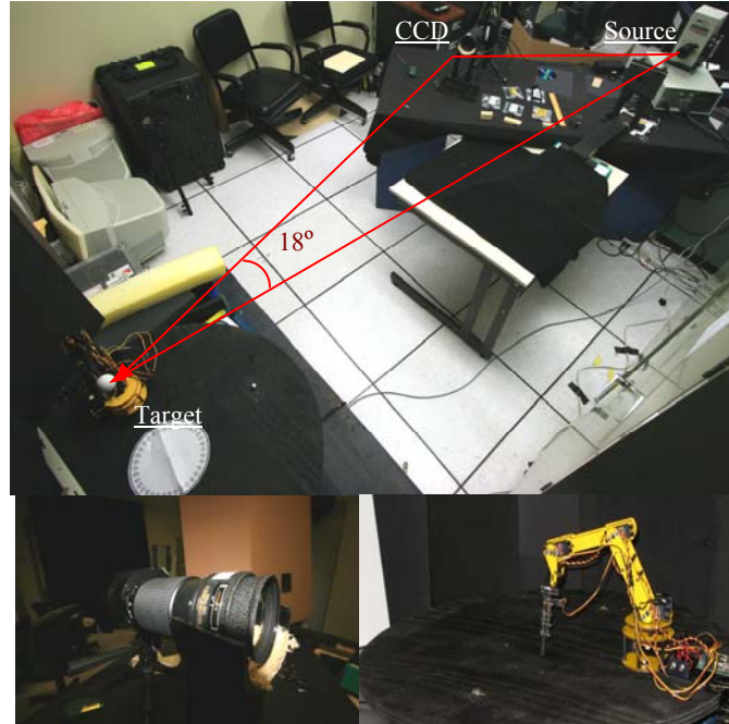
Fig. 2. Digital images taken on laboratory set-up and equipment. Top image: full laboratory set-up. Bottom left image: CCD camera with attached filter wheel and telephoto lens. Bottom Right image: close up on the robotic arm and rotary table.
