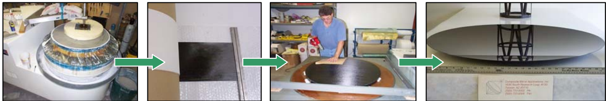
Figure 4 CFRP fabrication sequence from left to right, processing the glass mandrel, CFRP prepreg material, lay-up of prepreg over the glass mandrel, processing and release CFRP mirror from the mandrel, ready for coating.
