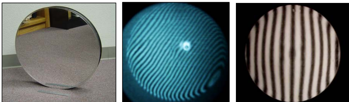
Figure 6 (Left) 0.4m parabolic CFRP mirror with aluminum coating, (Center) interference fringes for the mirror, (Right) 50lines/inch Ronchigram for mirror. Note turn-up edge [3] and central divot, indicating mandrel features.
