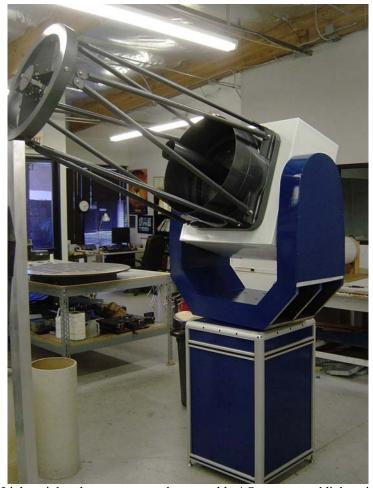
Figure 3- Lightweight telescope mounted on portable AO system and lightweight mount.
