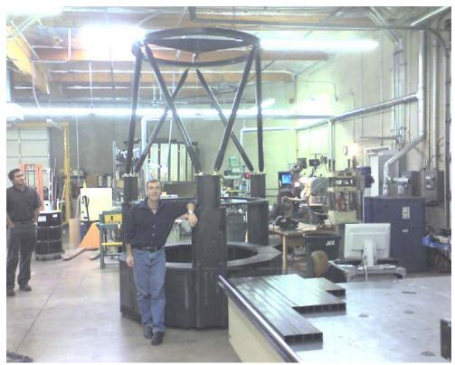
Figure 6- Picture of 1.4 meter telescope Optical Telescope Assembly (OTA).
