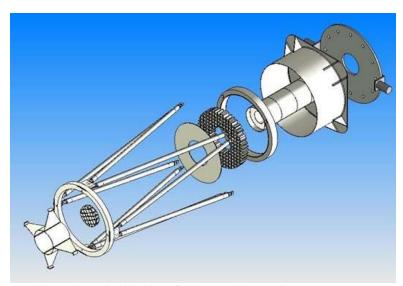
Figure 2: Exploded view of 0.4 meter CFRP telescope prototype
