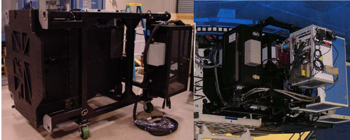
Fig. 6. Hokupa'a 85 (in the lab, left), one of the e85 element systems built at the IfA. It is an 85-channel adaptive relay designed to mount directly on the telescope (right). The APD enclosure is on the left side of the mounted instrument and the large blue box on the right side of the instrument holds the electronics for actuating the DM and for counting and processing pulses from the APDs.
