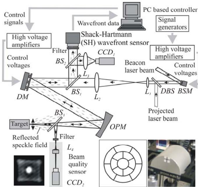
Fig.1. Scheme of the experimental setup used for closed loop experiments using SA PC and conventional PC. The image on the left is taken with the beam quality sensor where the scanning beacon laser and the laser spot of the projecting laser can be seen. The side length of the image corresponds to 120 micron. The two photos on the right show the 13-channel
