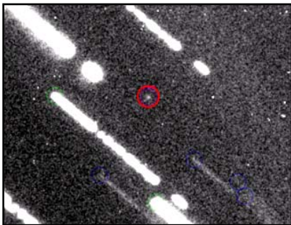
Fig. 2. Detection (see red circle) of potential Mars impacting asteroid 2007 WD5 (visual magnitude ~24). The image is composed of 42 stacked 2 minute exposures taken over a 1.5 hour period. The object was moving at 0.25 arcseconds/minute.
