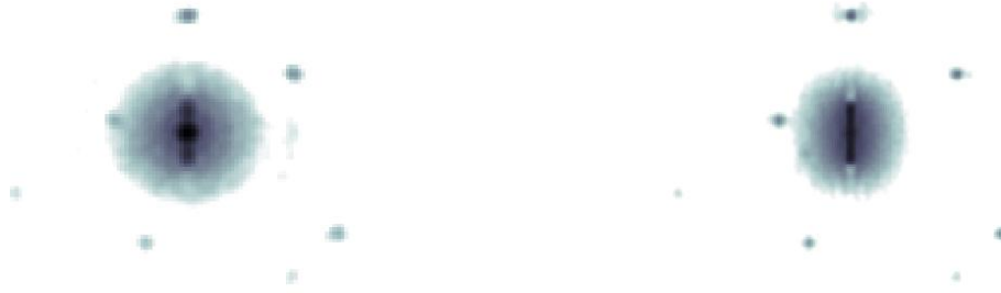
Figure 4. A demonstration of how the detection sensitivity is improved by extending the observation period. Here the restored images, at 0.88 \mu\text{m} (left) and 0.44 \mu\text{m} (right), are based on 77 seconds of simulated data including WFS and wavelength diversity measurements ( \sim 1,200 \times 256 \times 256 pixel images). The 25 \text{ cm} \times 25 \text{ cm} targets at a distance of 150 m from the main satellite are now identified with a high degree of confidence (i.e., the probability of false detection is low because the target is clearly detected at two widely separated wavelengths). The images are displayed on a logarithmic scale to emphasize the low-level structure.
