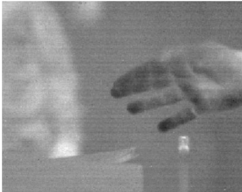
Figure 11. Corrected image from 320 x 256 pixel DWELL FPA
