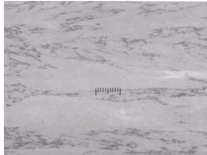
Fig. 9(a) Microstructure of CVD SiC
