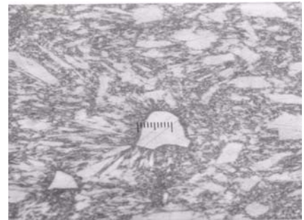
Fig. 9(b) Microstructure of Trex CVC SiC
