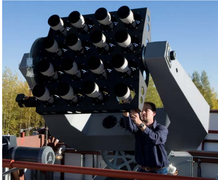
Figure 2. The second generation RAPTOR sky monitoring array. This array simultaneously monitors 10^3 sq-degrees with a sensitivity of R\sim 16^{\text{th}} magnitude in 30 seconds.
