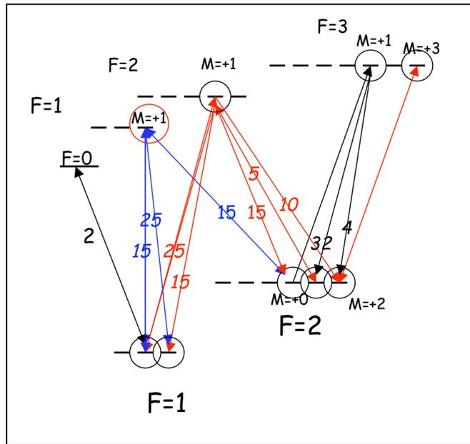
Figure 1: Simplified energy diagram of the Sodium D<sub>2</sub> transitions. The two ground states are separated by 1.771 GHz.
