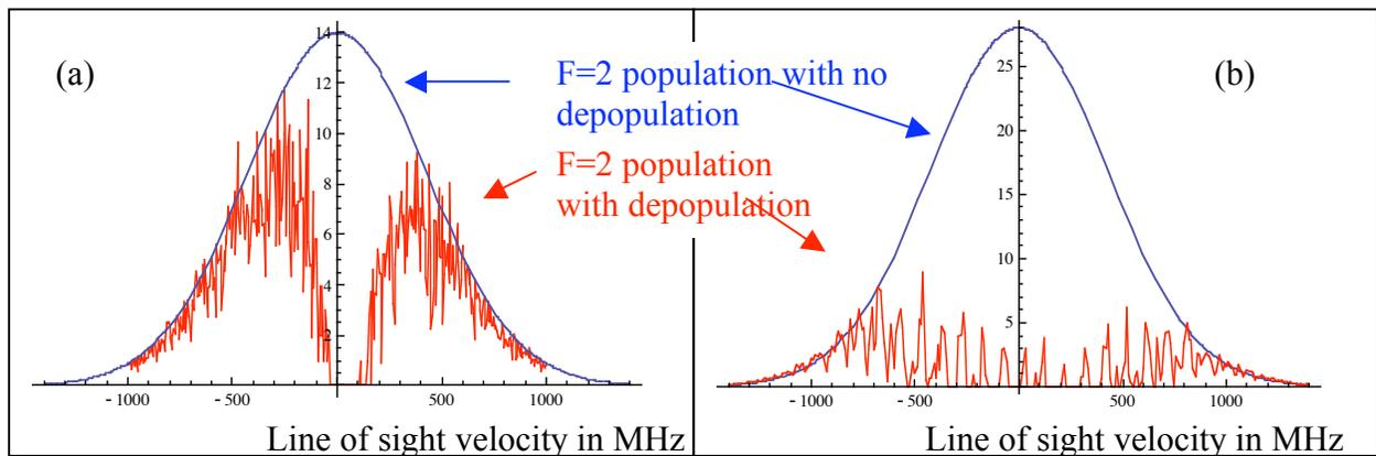
Figure 3: Population remaining in the F=2 ground state after a 100 μsecond collision lifetime for a laser intensity of 200 w/m<sup>2</sup>. These figures include the effects of radiation pressure, Zenith pointing, 0.5 gauss magnetic field at an angle of 30<sup>0</sup> to the laser beam. (a) is for a single frequency CW laser (b) is for a laser with lines spaced 98 MHz apart under a Gaussian envelop of 800 MHz FWHM.
