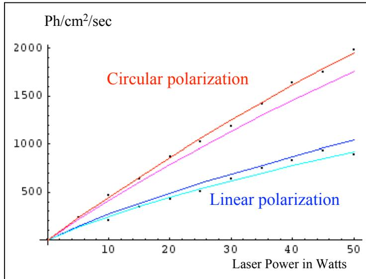
Figure 6: Calculated photon return on earth for the SOR laser assuming 2 arcsecond seeing and a column density of  $1.9 \times 10^{13}$  atoms/m<sup>2</sup>. Collision lifetime is 40  $\mu$ sec.
