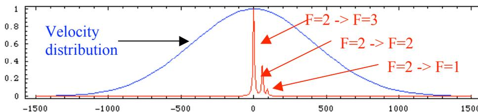
Figure 2: Doppler line of sight velocity distribution of sodium atoms in the mesosphere compared to the natural line width of the sodium D<sub>2</sub> line
