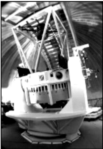
Fig.1. The Magdalena Ridge Observatory's 2.4-meter fast-tracking telescope. An instrument (an engineering CCD camera) is shown mounted to the right fork tine at the right Nasmyth port.
