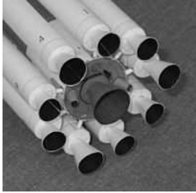
Figure 3. Scale model of a Delta 2 in the 7920 configuration. The three “air-start” solid rocket boosters, with their somewhat larger engine bells, are placed around the main engine at 120-degree intervals. Two “ground-start” boosters are placed in between each air start motor. Image copyright Erick Muñoz 2000-2008; used by permission.
