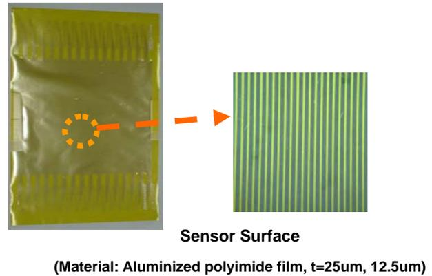
Fig. 2. An example of sensor prototype model
