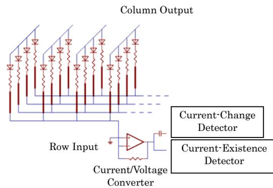
Fig. 3. Detecting circuit
