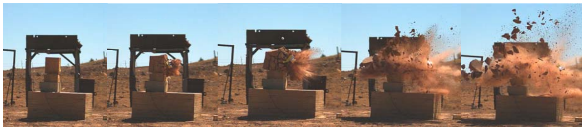
Fig. 4. The 1-foot cube target is shown as the impact progresses. The project is impacting the target from the right in the images.
