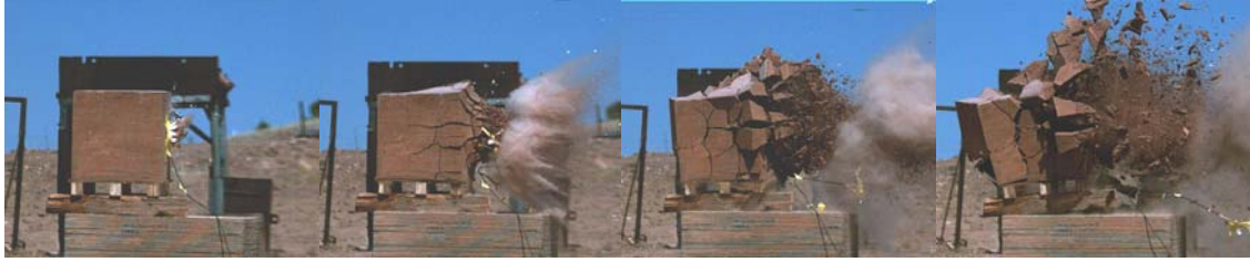
Fig. 5. The 2-foot cube target is shown as the impact progresses. The project is impacting the target from the right in the images.
