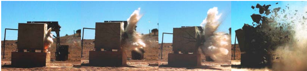
Fig. 6. The 3-foot cube target is shown as the impact progresses. The project is impacting the target from the right in the images.
