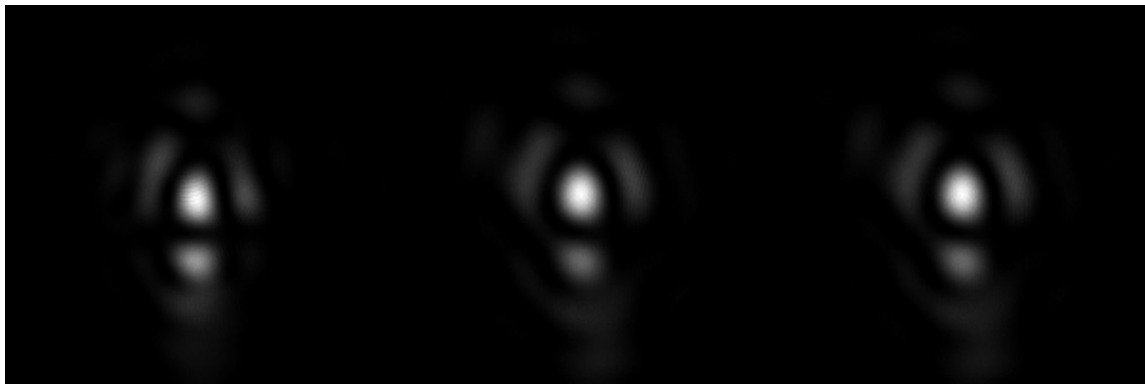
Figure 3: A schematic of the broadband corrected photon sieve telescope (top). Note that the final two mirrors are only used to produce a focus and could in principle be replaced by a single, smaller optic. The resulting experimental demonstration (bottom) shows a constant focal plane for 514nm, 532nm and 543nm light.
