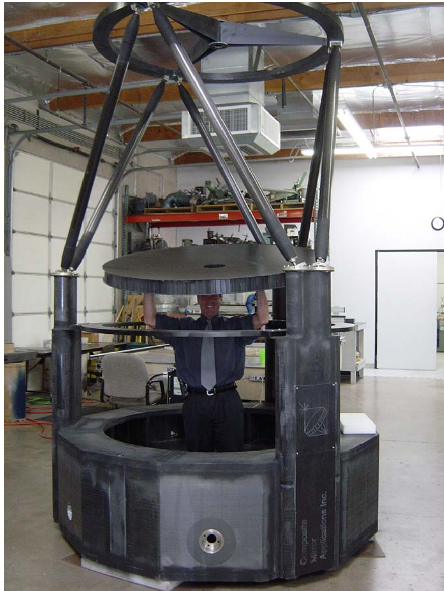
Figure 2. 1.4 meter CFRP telescope manufactured with optical blank. Final polishing of the mandrel will be completed soon and then the 1.4 meter primary mirrors can be replicated.
